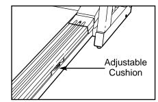
the cushions to level 2 or 1. It may be helpful to lift on the walking platform as you rotate the cushion. **Note: The faster you run on the treadmill, or the more you weigh, the firmer the cushioning system should be. Make sure that both cushions are at the same setting.**
